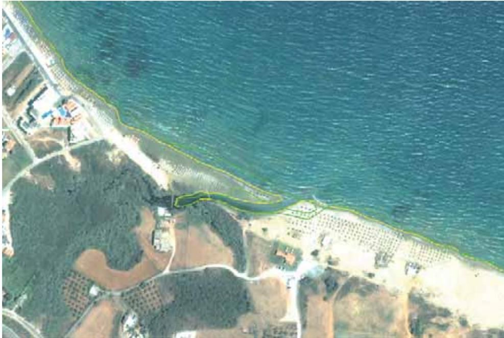
**Figure 14** - Part of the study area as a pseudocolour composition RGB: 3-2-1 of the orthorectified Ikonos image (scale 1:2000). The 1998 Shoreline is shown in green and the 2005 Shoreline is shown in yellow. A shift of about 50m to the ESE direction of the river outflow is observed.
