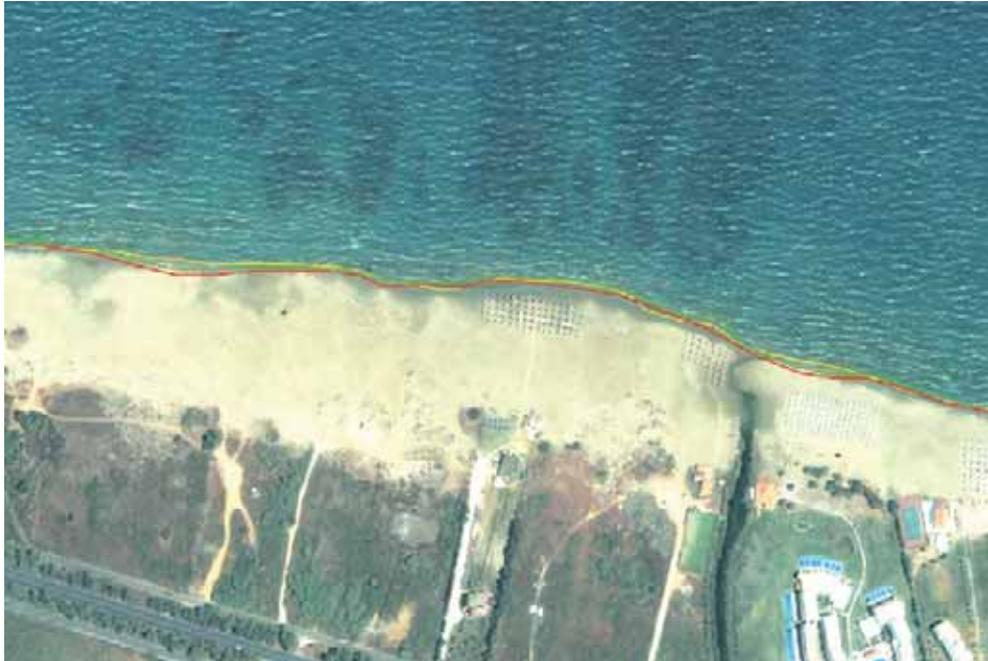
**Figure 13** - Part of the study area as a pseudocolour composition RGB: 3-2-1 of the orthorectified Ikonos image (scale 1:2000). The *in situ* derived shoreline is shown in red, the 1998 Shoreline is shown in green, whereas the 2005 Shoreline is shown in yellow.
