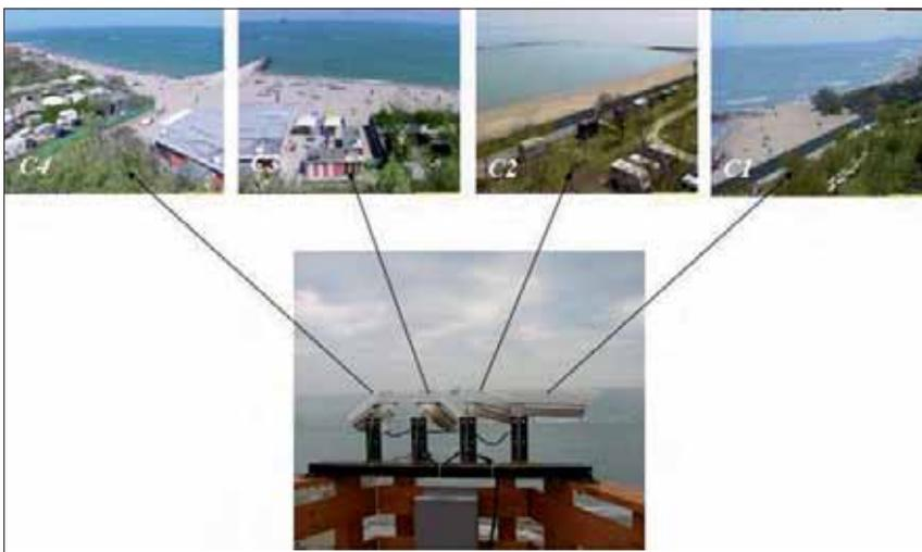
**Figure 4 - Lido di Dante Argus station - images taken by camera 1, camera 2, camera 3 and camera 4.**
