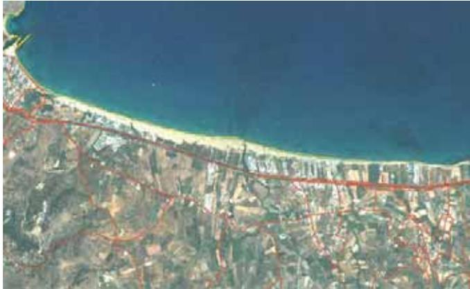
**Figure 7 - Pseudocolour composition RGB: 3-2-1 of the orthorectified Ikonos pan-sharpened image with the road network (red lines) and the shoreline extracted from the aerial image (yellow line) superimposed. Differences in shoreline between 1998 and 2005 are obvious.**
