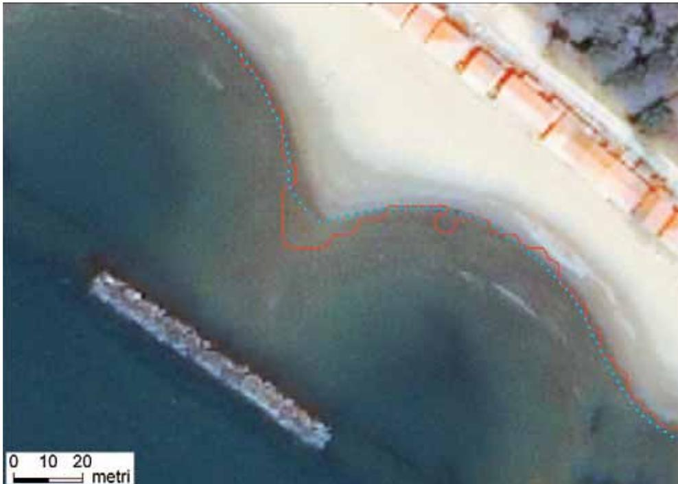
Figure 10 – Shoreline extracted from the B2/B4 ratio (in red); waterline from DGPS (in light blue). The distance between these two lines is larger in the zones immediately behind breakwaters, where beach slope is lower.
