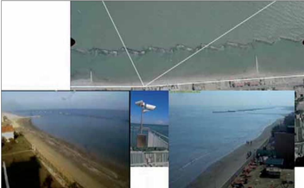
Figure 5 - The EVS SVM Video system. The left-hand side is a videocamera and the right-hand side is a still camera.
