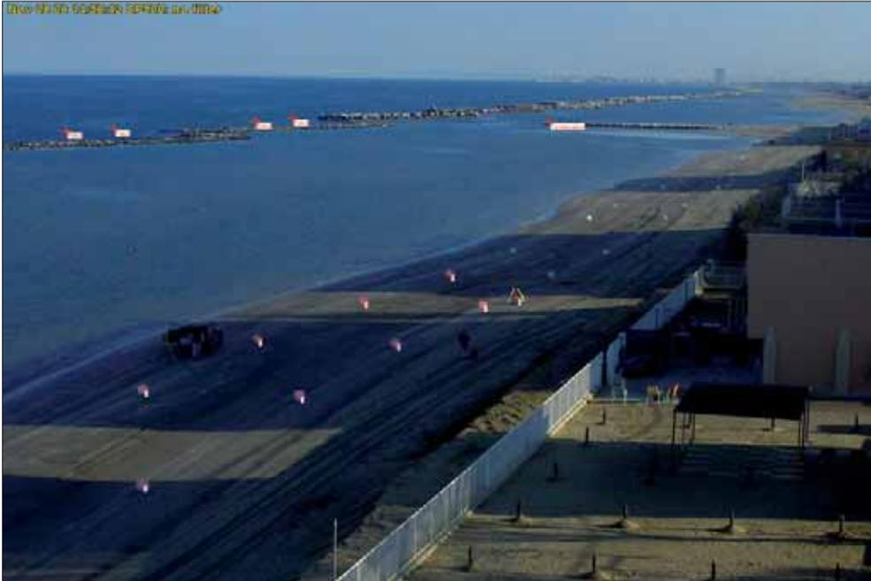
**Figure 3 - Timex image by still camera during the GCP survey with RTK-GPS in Igea Marina. The points show the GCPs location.**
