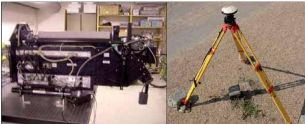
Figure 2 - LiDAR Hawkeye II system (left) and GPS station (right).
