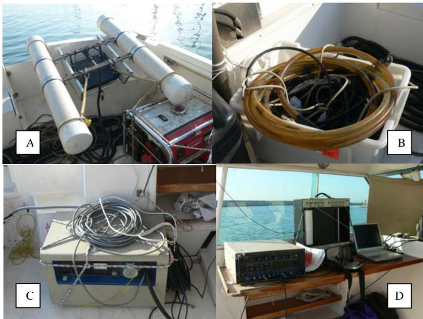
*Figure.7.* The basic seismic system includes different parts: (A) Boomer plate mounted on a Catamaran, (B) Hydrophone, (C) Power Supply, and (D) Receiver and EPC graphic recorder.
