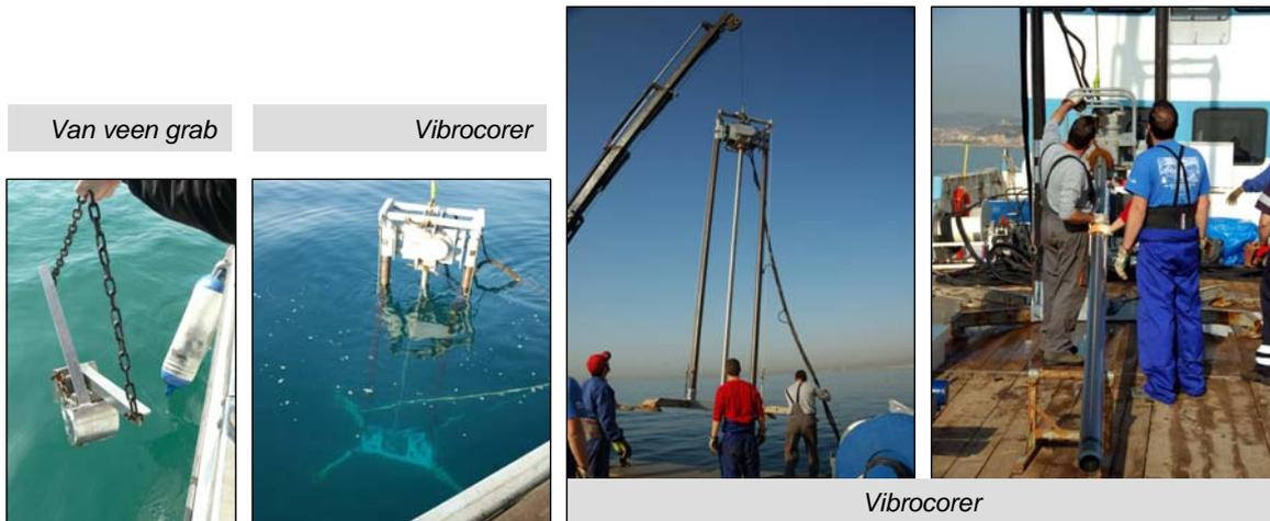
Figure 11. Image of a Van Veen grab and deploy of vibrocorer. After recovery, the vibrocorer can be rotated to a horizontal position to facilitate the removal of the liner.
