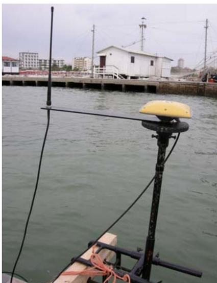
*Figure 3.3.* The bar supporting the “rover” station and the submerged transducer of the echo sounder
