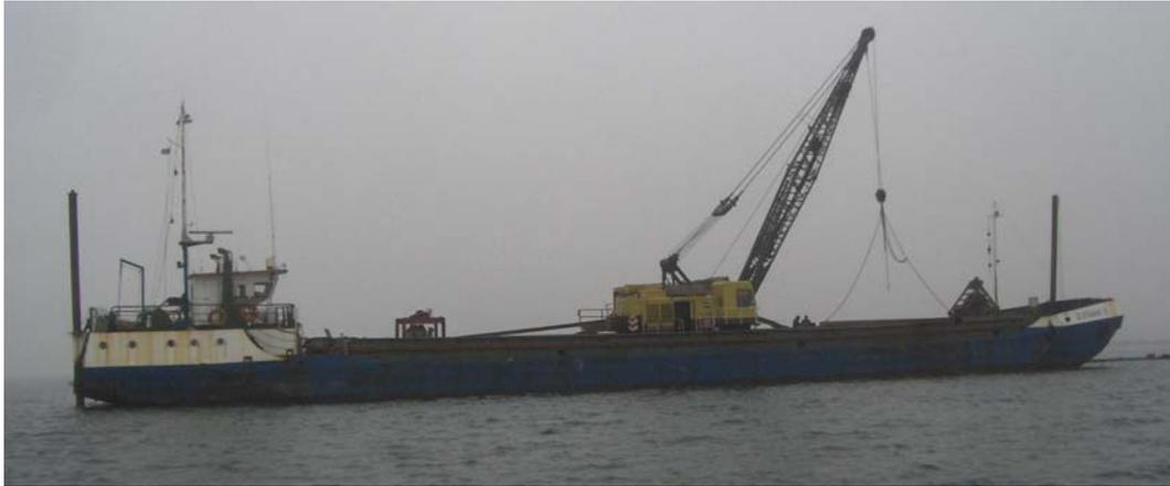
Figure 2.4. A barge used for sediment transport along the coastline of Emilia-Romagna
