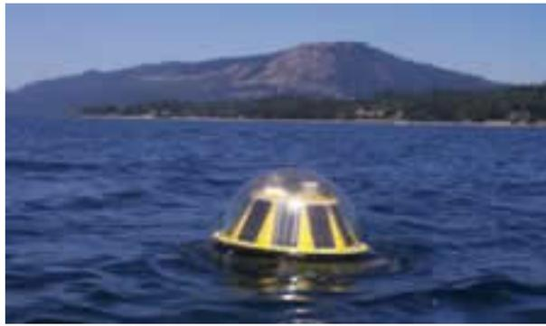
Figure 2: examples of a typical oceanographic station equipped with wave buoy
